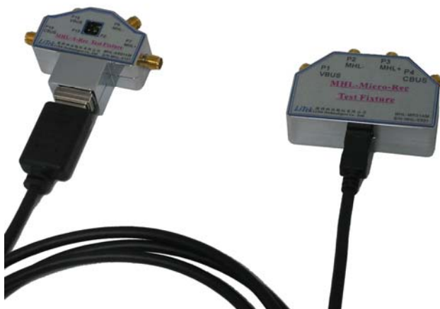
Fig2: MHL Cable plugged into LiTek's MHL Type A receptacle Test fixture and LiTek's MHL Micro USB Test fixture.
