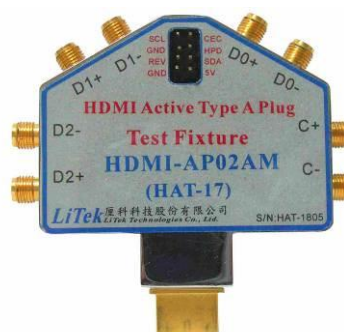
Fig3: HDMI-AP02AM, HDMI Active Plug Test Fixture
