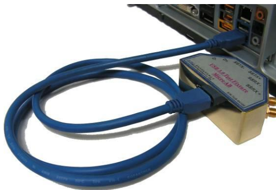
Fig2: USB3-MR01A plugged into Host Device after Type A to Type Micro A/B cable assembly
