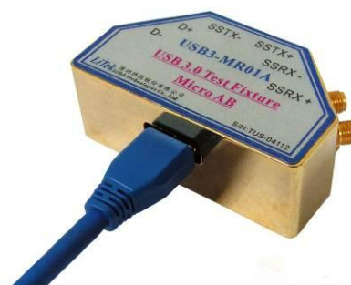
Fig3: USB3-MR01A plugged with Type Micro A/B Plug DUT.
