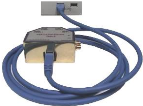
Fig2: USB3-BR01A plugged into Host Device after Type A to Type B cable assembly
