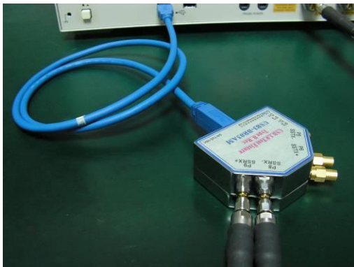
Fig2: USB3-BR03AM plugged into Host Device after Type B to Type A cable assembly
