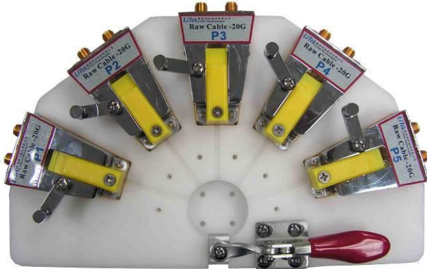
Fig 1: LT-100R-20G-5P Raw Cable Test Fixture Set
