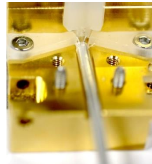
Fig 4: Twin-axial cable pressed on twin-groove
