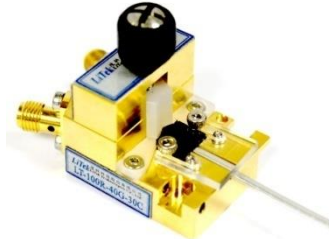
Fig 3: LT-100R-40G-30C with DUT
