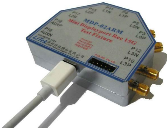
Fig2: Mini Display-port REC Test Fixture plugged With Thunderbolt Cable.
