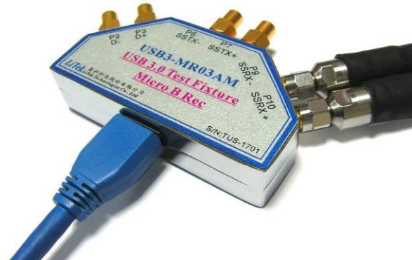
Fig3: USB3-MR03AM plugged with Type Micro B Plug DUT.
