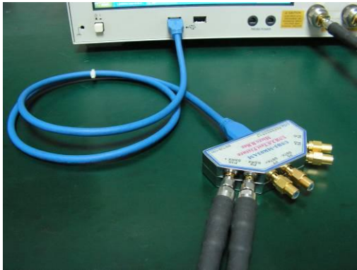
Fig2: USB3-MR03AM plugged into Host Device after Type A to Type A cable assembly
