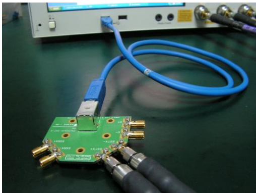
Fig2: USB3-BR03AR plugged into Host Device after Type B to Type A cable assembly
