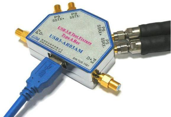
Fig3: USB3-AR03AM plugged with Type A Plug DUT.
