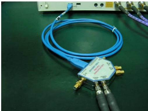
Fig2: USB3-AR03AM plugged into Host Device after Type A to Type A cable assembly
