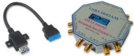
Fig3: USB3-IR02AM plugged with USB3.0 Internal DUT.
