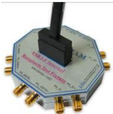
Fig2: USB3 Internal Cable plugged into USB3-IR02AM Test Fixture.
