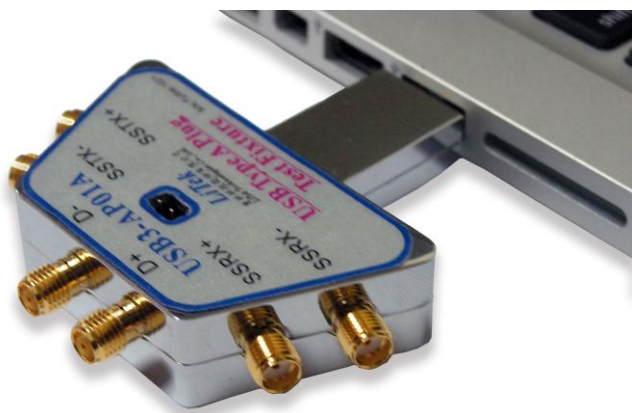
Fig2: USB3-AP01A plugged into Host Device
