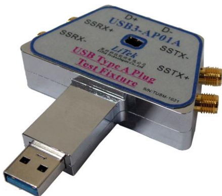
Fig1: USB3.0 Type A Plug Test Fixture (USB3-AP01A)
